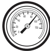
Attach air hose. Be sure line pressure is 80-100 PSI. (Pressure adjustment may be needed depending on framing material density)
