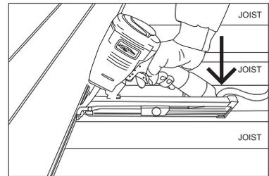
Once fastener is fully inserted, apply pressure to disengage the safety. **Then** lower the back of the gun allowing the magazine to sit on the support joist to assure correct angle, and pull the trigger.
