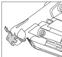
With horned tab points outward insert the opposite tab into the nose of the gun.
