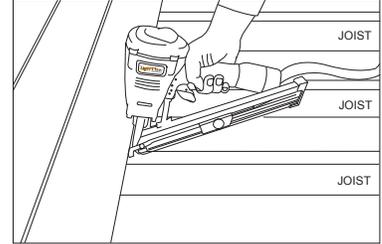
Holding the gun upright, insert the horned tab into the groove of the deck board directly over the support joist.
