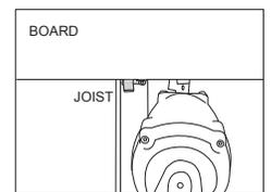
With the magazine still resting on the joist, slide the nose of the gun to the right removing it from the attached fastener.
