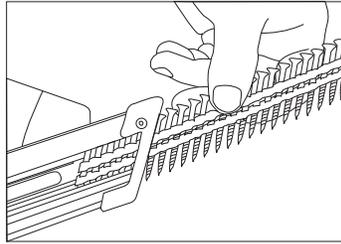
Insert a sleeve of collated pneumatic screws into the rear of the magazine.
